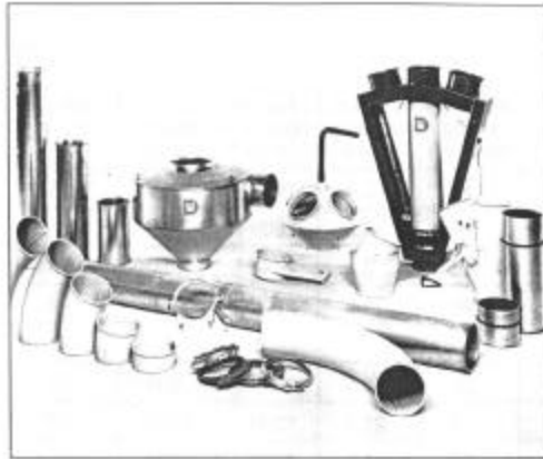
The pipe system comprises a wide range of straight pipes, bends, diverters, hoppers, cyclones, suction heads, etc. Assembly is effected by means of the patented OK quick-release couplings without the use of tools. See special brochure.
